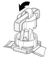
2. Turn Counter Clockwise Until All Twist Are Removed. Pull Straps From Both Sides to Reseat Handle
